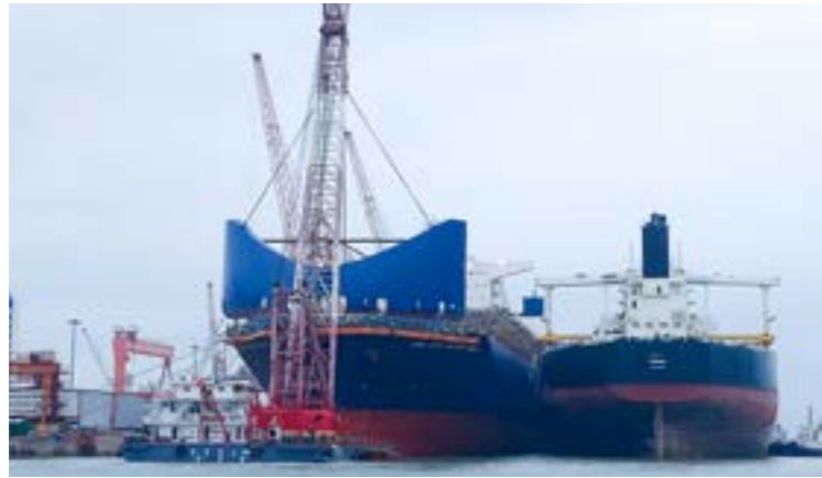
"The CMA CGM Marco Polo is equipped with a new wind deflector installed on its bow. This new equipment improves the ship's aerodynamics and should reduce fuel consumption by 2%."
